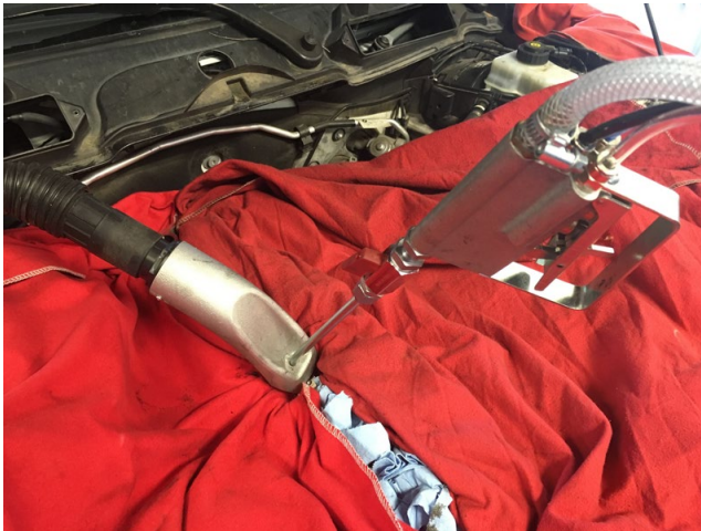
Using carbon blaster on swirl port.
