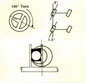
3) Slightly Harder Turn. About two-thirds of a turn on the steering wheel rotates the slider pin to the 12 o'clock position. Note that even though the front wheels are still turning, the rear wheels are centered again.
