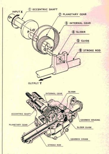
first is a schematic view. It is hardly drawn to scale, but it makes the relationship of the moving parts easier to visualize.
