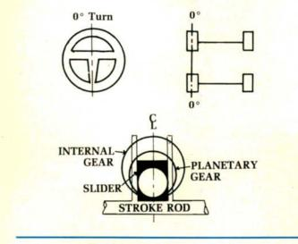
2) Gradual Turn. At less than half a turn of the steering wheel we see the rear wheels steering with the fronts. In the side view of the steering box, note that the rotation of the planetary gear has caused the slider pin to move to the 9 o'clock position. This has caused the slider to move to the side, moving the stroke rod laterally.
