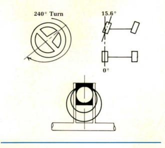
4) A Really Hard Turn. We've turned the steering more than one complete revolution at this point. Note that the slider pin is now at the 3 o'clock position. This puts it to the right of the center line and reverses the movement of the stroke rod. As you can see, the rear wheels are steering opposite the fronts at this point.
