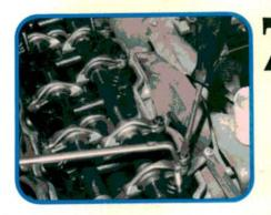
Don't overtighten those lock nuts or you'll pull threads. This will make the next adjustment very difficult when the adjusting screws want to turn with the nut. Just snug them down, and then double check the clearances to be sure they didn't change.
