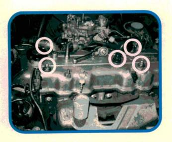
First, warm up the engine to warm—not blistering hot. Remove the air cleaner, cover the carb throat, and wash away as much grime as possible. Remove the valve cover and see if the cam followers are too hot to touch. If so, let them cool slightly.
