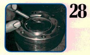
The inner race also goes on a certain way. This chamfer is cut to help you start the joint on the shaft. As a result, it will face away from the transaxle. In other words, the relief on the outer race and the chamfer on the inner race, face in opposite directions.
