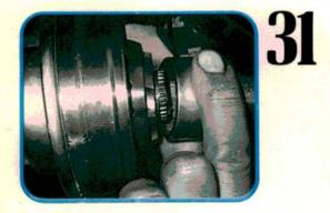
Here we are reinstalling the joint on the axle. The relief in the outer race will face toward the axle stubs. Start the snap ring over the splines with snap ring pliers and then drive it home with a small piece of pipe or a socket that just clears the axle splines.
