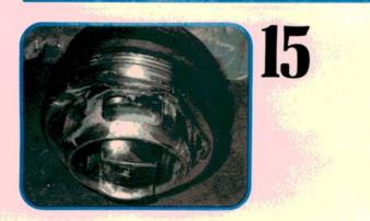
Here's a view of the Rabbit joint. It comes apart just like the Nissan one in the previous photo. You may have to wiggle the inner race and cage a bit the first time you try this, but once you get the knack, it's easy. Check that inner race for pitting, galling, and wear.
