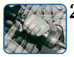
To install an internal snap-ring type joint on the axle, you'll need to enlist the help of a large persuader. Make sure you start the joint on the splines and whack it with a dead-blow or other type soft-headed mallet. Speaking of softheaded, I'm not holding the joint straight enough.
