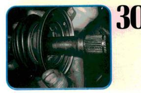
Slide the boot over the axle shaft and put a little grease in the bottom. This grease won't do a lot for the joint, but it will help seal the neck of the boot and keep water out. Don't install the boot clamp until the joint is on so you can turn it to align the bolt holes.
