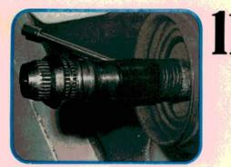
With the joint removed you can see the preload spacers. Between them is the groove for the snap ring. Later models use an internal snap ring. We'll cover this general type in the next picture. Internal types have the groove at the outer end of the shaft.
