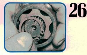
With that clip removed, the outer race slides off easily. The Nissan joint also has a small retaining clip on the back. Remove it and tap the joint off for cleaning and inspection, or replacement. The same cautions apply to this snap ring as they did for the Rabbit's.
