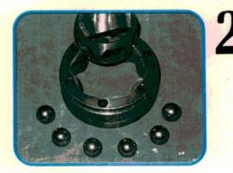
This joint looks good after clean up. The ball bearings are shiny, the races smooth, and the cage sound. Look for badly discolored or blued ball bearings, abnormal wear at the cage/ball bearing contact surfaces, and any signs of scoring, galling, breakage, or excessive wear.
