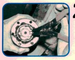
The outer joints were the tough part. The inner ones are really easy. The Rabbit-style inner joint is held to the axle by a circlip. Always replace this clip and put the face with the sharp edge facing inboard. With the clip removed, tap the joint to remove it from the axle.
