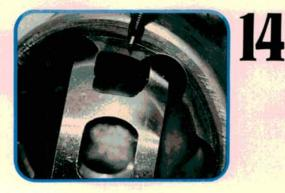
Here's a better view of one of the long windows in the bearing cage. Another long window is located directly across from this one. If (and only if) you align the cage with the outer race of the joint, you can remove it completely. Check the cage for signs of wear or damage.
