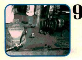
Mount the axle in a soft-jawed vise for disassembly. The metal collar on the boot for the inner joint can be stubborn. It's nothing a small chisel won't handle. If you're replacing the outer boot, save some time and just cut it away, clamps and all.
