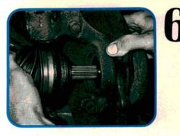
See the split in the ball joint pinch collar? We caution you again not to spread it too far when trying to remove the ball joint. It's pretty tough stuff but it does have its limits. If you're only being paid to replace a torn inner boot, don't cut the outer one on the strut tube.
