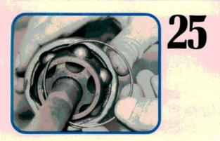
The joint on the Nissan is slightly different. Remove the boot and clean away enough grease to expose this retaining clip from its groove. This ring is hard to see when it's covered with grease and you'll wonder why the darn thing won't cooperate.
