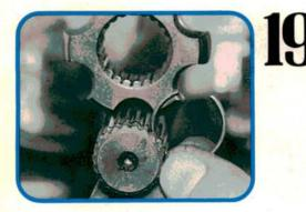
This little clip doesn't look like much does it? Well, it can be incredibly obstinate. The ring expands to a size slightly larger than the diameter of the splines and locks in a companion groove cut into the inner race. To remove the joint, you have to compress or cut the ring.
