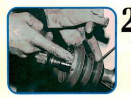
Slide the inside clamp over the axle. Then slide on the boot. Install the preload washers. Put a fingerful of grease on the base of the boot to help seal it. Now we're ready to pack the joint with the grease in the kit and reinstall it. Don't forget to tighten the clamps.
