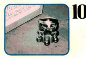
With the outer boot out of the way, clean away enough grease to expose the spreadable clip holding the joint on. Spread it with pointed snap-ring pliers and tap the joint off with a soft mallet. This photo shows the clip right above the ball bearing closest to you.
