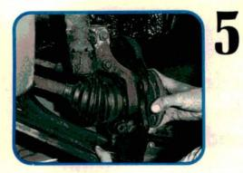
Pull down on the control arm and pull the drive hub away from the outer drive joint at the same time. The outer joint splines are not a press fit in the hub, but you may need a little penetrating oil on them and on the ball joint in order to finally free things up.
