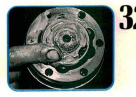
Before you pull the boot up tight, pack the joint with the fresh grease that should be supplied with the boot kit. Work the grease into the joint as you would with a wheel bearing. Use your fingers to pack the joint and be sure you remove all the air pockets.
