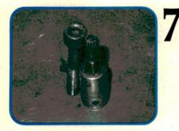
Since the inner joints bolt to the transaxle drive stubs on the Rabbit, you'll need this splined socket to remove the bolts. Take the time to clean the bolt sockets. The teeth are very fine, and unless the socket gets a good bite, you'll strip them in an instant.
