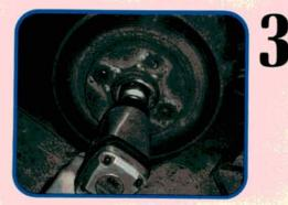
Take your impact and loosen the axle nut. If you're using the Armstrong method and a breaker bar, you'll want to do this while the car is still on the ground (tire installed, brakes on). In the best of all possible worlds, this nut should be replaced and torqued at reassembly.
