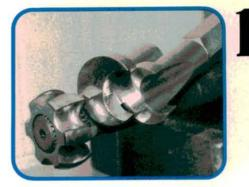
These drivers from Stempf Automotive come in two different sizes for large and small axles, and have an interchangeable extension handle to keep your knuckles out of harm's way. We cheated a little and disassembled the joint first so you could see where the driver rides.
