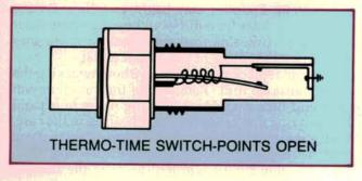
As a result, we have crank voltage and ground supplied to the heating coil and the cold start injector. The heating coil warms the bi-metallic spring causing it to deflect slightly. This movement opens the points, eliminating the ground circuit to both the switch heater and injector.
