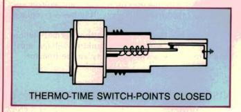
The same current used to energize the starter solenoid in the crank position also feeds the time switch and cold start injector. It travels to the cold start injector to energize it. It also travels through a heating coil wrapped around another bi-metallic spring, similar to the one found in the control pressure regulator. A set of contact points on the bi-metallic arm connect it to ground. Ground is also supplied to the cold start injector as long as the points in the time switch stay closed.
