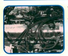
Run the engine up to operating temperature before removing the valve cover. This engine seems to cool off very quickly. Valve clearance increases about .002 inch (.050 mm) from cold to warm. If the engine cools too much during your adjustment, the last valves that you do will be too loose.
