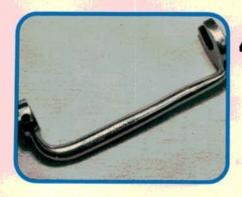
A tool such as Kent-Moore's or Snap-on's (shown here) will get your ratchet up above the cam and keep your knuckles away from sharp aluminum edges. Tool also works on pre-1980 200 SXs and 510s with the L20B engine. If you don't have the tool, a 17 mm open end will do all but the number one exhaust.
