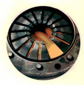
This clutch was noisy or didn't work smoothly. Ignore the missing piece of diaphragm. See the deep groove the release bearing has worn into the diaphragm? This tells you the release bearing is seized up, seizing up, or it's sticking on its sleeve. Check for a dry, worn, or burred sleeve.
