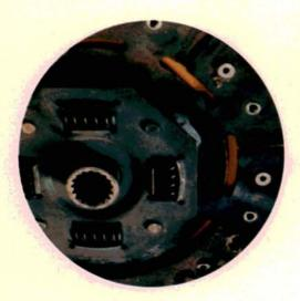
Broken disc lining can be caused by driver error such as driving too long in the wrong gear. Over-revving can also cause it. This means that when the driver pushed in the pedal, the rear wheels drove the clutch faster than it wanted to rev.
