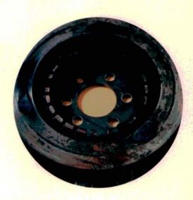
If the clutch has slipped or chattered long enough and severely enough, deep wear grooves and/or hot spots form on the pressure plate. Check the pedal's free play. Insufficient free play is a major cause of slippage and clutch/pressure plate overheating.
