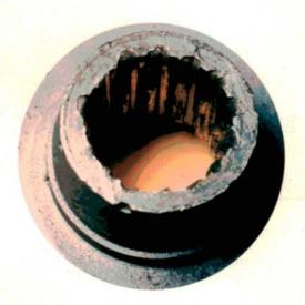
The clutch may chatter or may not disengage. The trans may be hard to shift. Stripped splines suggest damaged or badly worn trans splines or trans-to-engine alignment problems. The pilot bearing may be missing or severely worn. Or, some gorilla may have forced the input shaft into these splines.
