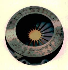
Clutch chatter, accompanied by severe chatter marks on the pressure plate, are often caused by oil or grease contamination. But the pressure plate itself may be warped. And don't overlook soggy, split, or loose engine or transmission mounts. Also watch for sloppy universals or CV joints.
