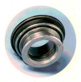
On this type of release bearing, a shiny wear ring around the backside of the bearing tells you to check for a worn clutch release fork. Remember to inspect the point where the fork pivots—or attaches to its pivot—for wear, dryness, or cracks.
