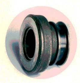
The more a clutch slips, the more heat it creates. An overheated clutch usually destroys the clutch release bearing. In the worst cases, the bearing will have this burned or carbonized appearance. Don't risk the clutch job. Replace the release bearing as part of the clutch job.
