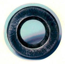
This swirl or spiral pattern on the front of the bearing suggests a trans-to-engine alignment problem. Alignment dowel pin problems aren't too common. However, it only takes a moment to inspect both the block and bellhousing for signs of a missing dowel pin.
