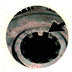
This clutch won't disengage smoothly and freely. This clutch is noisy. There's tapered wear on one side of the clutch splines. This is yet another example of a trans-to-engine alignment problem. But there's also a chance the pilot bearing's severely worn.
