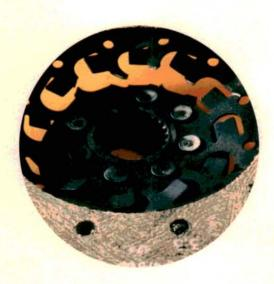
The guy changed his own clutch but then he couldn't get the car out of the driveway. You tow it in, take it apart, and find one side of the clutch hub is cracked away. Poor quality? No, the guy let the transmission hang down unsupported and the weight of the trans damaged the clutch.
