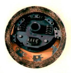
A severe trans-to-engine alignment problem can tear the damper completely out of the clutch plate. Maybe someone pinched a cable or wiring harness between the bellhousing and the block. Maybe someone forgot to install the pilot bearing—or just overlooked a severely worn one.
