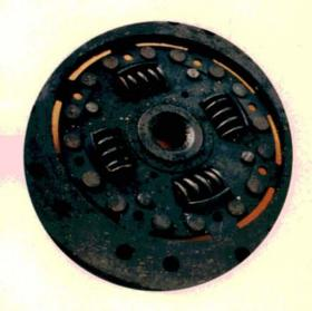
A clutch disc that's overheated due to slippage may have this charred look to it. If an oil leak caused the slippage, the disc'll probably still be oily. Always clean the clutch dust from the bellhousing and flywheel. Severe buildups of clutch dust can actually cause grabbing and/or chattering problems!
