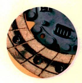
The disc's fairly new, but it's already slipping or chattering. Whenever the disc lining's worn only in the center or only on the edges, you know the flywheel has to be resurfaced or replaced. Sometimes, you ignore a marginal flywheel and get away with it. Other times, you don't get away with it!
