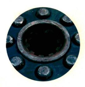
The clutch doesn't engage or disengage smoothly. Rusted splines confirm that either the transmission splines weren't lubed or they weren't lubed with the right grease. Use moly grease or white lithium grease. Slide the disc on and off the lubricated splines and then wipe off any excess grease.
