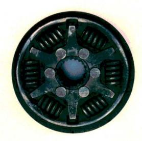
After a while, your otherwise-thorough clutch job has started to slip, grab, or make noise. The car has a stepped or recessed flywheel? Those shiny wear marks on the damper tell you that the machinist ground one flywheel surface instead of two. Now the flywheel's clutch recess is too shallow.
