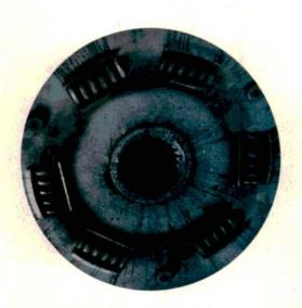
The new clutch begins slipping and/or chattering. This grease splatter tells you the installer slopped too much grease on the trans splines. All the splines need is a film of grease. And don't over-lube the pilot bearing, either! Also watch out for leaking or missing seals on the pilot bearing.
