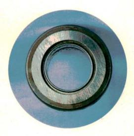
This outside wear pattern on the release bearing suggests mismatched parts. The installer used a thinner-than-original disc. However, a perfectly good replacement clutch set may not always look identical to the parts you removed from the car. Your supplier has got to be on the ball!
