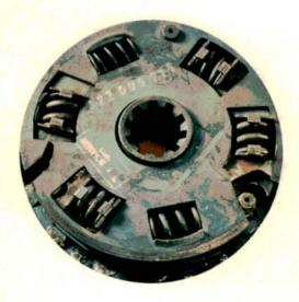
The complaint is a noisy clutch. You find that the damper cover's been torn off the damper. Odds are, this driver's too lazy to downshift. He lugged the engine down in high gear one time too many. Here, the debris may wedge itself on one side of the disc or the other and then jam up the clutch.
