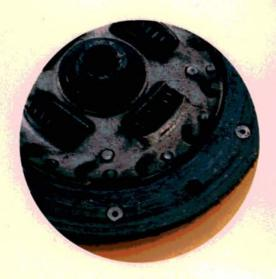
Depending upon the vehicle's mileage, this could be normal wear. But if the disc lining's down to the rivets at relatively low miles, it could mean driver abuse. It could also mean that the guy who installed the last clutch didn't replace the pressure plate when he should have!
