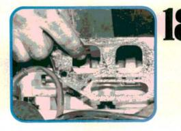
Pay attention! You can reverse this intake gasket and all the intake bolts will still go in unobstructed. You may not realize you reversed the gasket until the job's all buttoned up and coolant is gushing out of the engine!
