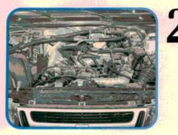
No question, the easiest, fastest way to do this job is to remove the hood. Thankfully, you just disconnect the washer hose, remove two bolts, and lift off the 900's hood. No, there's no adjustment to worry about—just reinstall those two bolts.
