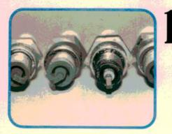
When a head cracks, the plug inside the cracked chamber will be cleaner than the other plugs—usually white. The plug will also be wet with coolant.
