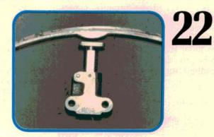
If you have to replace a chain tensioner on an H-series Saab engine, always install this updated tensioner (P/N 8817405). If that engine has Torx<sup>®</sup> -head head bolts, odds are it's already equipped with this style of timing chain tensioner.
