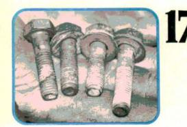
These bolts hold the exhaust manifold flange onto the turbocharger. The one longer bolt on the right goes into the upper *inboard* flange hole.
