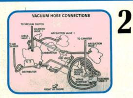
The underhood decal is a good source of emissions information if you don't have a manual. It gives a good idea of where things are located on the engine. Check for proper hose routing. Also look for dry or cracked hoses at this time.
