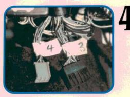
Under the dash are test connectors 3 and 4, which are red and black. These offer access to certain feedback components that (underhood) connectors 1 and 2 do *not*. To prevent damage to the wiring terminals, always probe these connectors from the wiring harness side of the connector.
