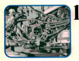
There's a lot more here than on the old VW! Subaru used three different emissions systems during the 1983 model year: a Hitachi two-barrel, a Hitachi two-barrel with feedback control, and a Carter-Weber with feedback control. Find out what you're working on before you go too far.
