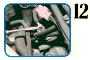
A thermal vacuum valve mounted on the left side of the engine controls application of vacuum to the distributor advance and the EGR valve. The ECM also provides vacuum control through a vacuum solenoid. If you have vacuum problems, check these valves for proper operation and correct hose routing.
