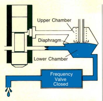
Here's a closer, more simplified look at the frequency valve's effect on the fuel distributor. When the frequency valve is closed, the lower chamber pressure is greater than the upper chamber pressure. This greater pressure pushes the diaphragm upward, restricting the fuel outlet port to the injector.
