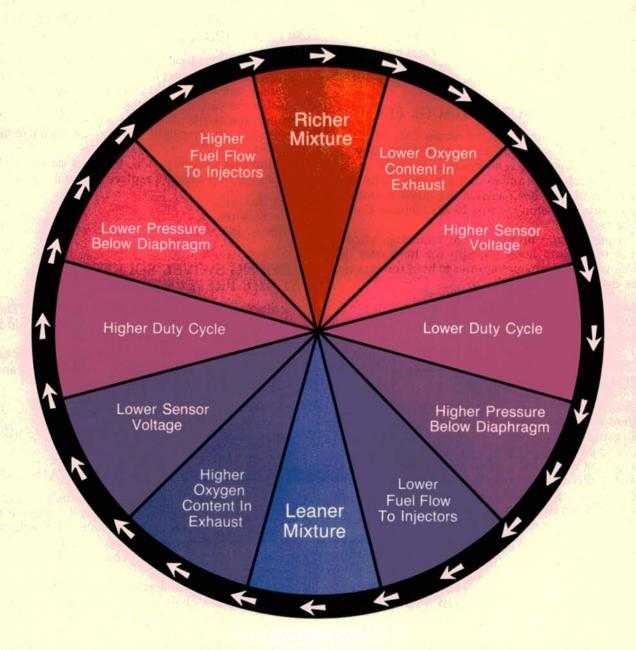
Remember that once the ECU gets a signal from the oxygen sensor, the ECU makes a command to correct the mixture condition. If you follow the actions and reactions around this chart, you'll get a feeling for how a closed loop feedback fuel system works.
