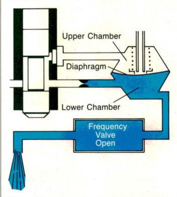
When the frequency valve opens, it reduces pressure in the lower chamber. Then the spring in the upper chamber pushes the diaphragm downward and increases the opening at the fuel outlet port. This increases fuel flow to the injector. The more fuel the injector receives, the richer the mixture becomes.
