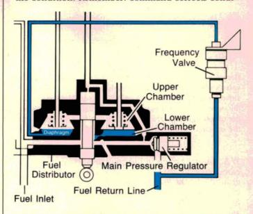
This schematic shows how the frequency valve is tied into the normal K-Jetronic fuel distributor plumbing. When the ECU grounds one terminal of the frequency valve, the valve opens. With the valve open, some of the lower chamber fuel pressure vents back to the fuel tank.
