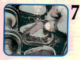
Always replace these seals that seal the valve cover to the top of the spark plug wells. The seals tend to dry out and crack. Then the plug wells fill up with oil. Check with your supplier beforehand, because all valve cover gasket kits do not include these seals.
