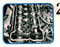
The driver-side or carburetor-side cam is the intake cam. Some guys prefer to adjust the valves one camshaft at a time. They say this minimizes the chances of you making a mistake. Mercedes recommends that you set the valves cold.
