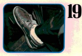
After reinstalling the caliper, bleed any air from the system. To dislodge all the air bubbles, sometimes you have to lightly tap the caliper. Once you've bled out the air, the piston should move out to meet the brake pad.
