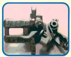
Once you've taken the caliper off the car, take the time to clean it thoroughly. A little extra time spent here will make the job easier later. Look the caliper over carefully. Make sure it's a good candidate for an
