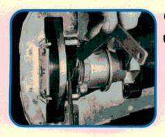
If the pads are worn thin, the primary piston (the one next to the rotor) will be screwed out pretty far. Before exercising the caliper, use Saab special tool 8996043 or equivalent to partially screw the piston in. Turn it clockwise and be careful not to damage the caliper boot.
