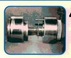
Here are the brake pistons removed. See how they screw apart to compensate for pad wear? You want to screw that primary piston (left) inward enough to keep it from popping out of its seal when you begin exercising the caliper in the next step. Always check for torn boots or rusted pistons.
