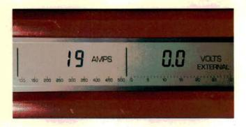
You need a bionic memory to remember which alternators need an external ground and where these grounds are on the car. If the charging system's misbehaving, don't worry about them unless the ground circuit flunks a voltage drop test. Clip one voltmeter lead onto the alternator case, clip the other lead onto the negative battery post. Then load the alternator. If the voltage drop's greater than about 0.3-0.4 volt, try grounding the alternator temporarily with a heavy jumper wire.
