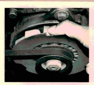
For a quick, convenient tension check, grab the pulley (where possible) and try to turn it by hand. If you can spin the pulley inside the belt, you know the belt's too loose. Also, watch the ammeter when you load test the alternator. If the output reading peaks and then suddenly drops off, you can bet the belt is loose!
