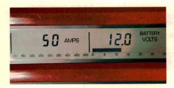
Ideally, you should check alternator output at a specified voltage and RPM. However, you can usually do a decent output test by running the engine at 2000-2500 RPM and loading the battery down to 12.0-12.5 volts. If your engine analyzer does a cranking compression test, it may help you get a quick-and-dirty output measurement. At the end of this test, shut the key off. Wait a moment. Then start the engine, floor the gas pedal, and watch the alternator output reading on the analyzer's ammeter.
