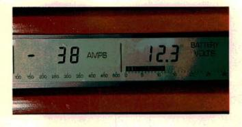
Sometimes you suspect that someone's installed an under-capacity alternator on the car. Okay, turn the key switch on (engine off) and turn on as many accessories as possible. Don't forget the air conditioner and the rear defroster! When the ammeter reading peaks, shut everything off. This total accessory drain shouldn't exceed 75 percent of the alternator's output. Here, I measured 38 amps total drain. That turned out to be exactly 75 percent of the alternator's 51-amp peak output!
