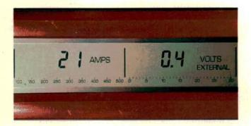
Because I've seen stupid voltage drops create so many bizarre charging system problems, I routinely voltage drop every system I test. Clip one voltmeter lead to the alternator output terminal, clip the other to the positive battery post. Load the alternator. A charging system can usually tolerate a 0.3-0.4 volt loss between the alternator and battery. If you measure a serious voltage drop here, trace the output wire until you find the cause.
