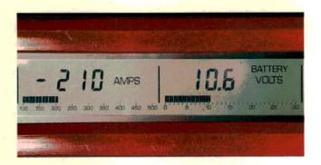
Load-testing is the quickest, most accurate way to isolate a weak or under-capacity battery. Sure, hydrometer readings can be helpful. But only a load test tells you how that battery will perform when you put it back in the car. Load the battery to half its coldcranking amp (CCA) rating for 15 seconds. If you don't know the CCA rating, a 190-200 amp load is usually a good starting point. A marginal battery not only makes the car harder to start, it also taxes the alternator.
