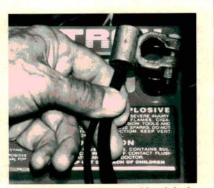
Never, ever remove a battery cable while the engine's running. Removing a cable removes the normal electrical load from the charging system. Once you've removed the cable, the charging voltage could skyrocket to several hundred volts before the voltage regulator has a chance to shut down the alternator! That voltage can do incredible damage to the electrical system as it races around trying to find a good ground.
