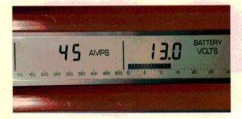
Load-testing is the safest, most accurate way to check alternator output. Loading the battery lowers battery voltage. Until you lower the battery voltage, the voltage regulator won't tell the alternator to charge! Fullfielding an alternator (bypassing the regulator) and snapping the throttle is both an inaccurate and risky output test. This approach can create dangerously high voltages that damage on-board computers or burn up accessories on the car that you forgot to shut off!
