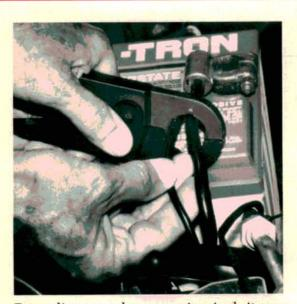
Depending upon how a car is wired, it may be difficult to get the ammeter pickup around just the alternator output wire. Clip the pickup around the wires that merge into the positive battery terminal. Turn the key on, note the ignition draw. If it draws six amps, add six amps to the output reading when you load test the alternator.
