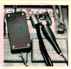
Want to safely and accurately read key-off drain with-a digital VOM? Then fabricate a resistor such as the one we showed you in the March Import Service (page 42). Or, purchase one from Interstate Batteries. After you connect this resistor in series with the negative cable, connect your VOM across the resistor. A 0.05-volt reading here means there's a 50 milliamp drain. Any drain less than 50 milliamps is okay.
