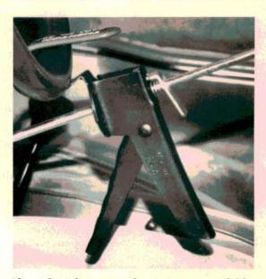
If you don't have any other test specs available, check alternator output at 2000-2500 RPM. I needn't tell you that on many of these engines, you can't reach the throttle linkage easily unless you remove the air cleaner. When the engine's scalding hot and the throttle linkage is hard to reach, I use an adjustable prop such as this one to hold engine RPM steady for me.
