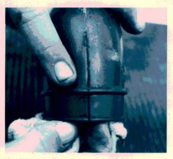
Watch out for small cracks that cause air leaks in the long plastic duct. This duct connects the air flow sensor to the throttle valve assembly.
