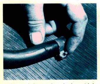
Auxiliary air valve hoses can also crack and cause air leaks. Remember that if an auxiliary air valve hose collapses, the engine will tend to stumble and stall when it's cold.
