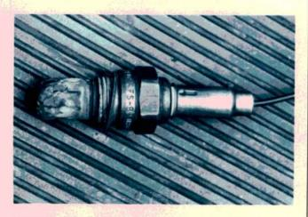
Silicone vapors ruined this oxygen sensor. Careless, excessive use of silicone sprays or certain silicone (RTV) sealers can cause this. Silicone contamination makes the sensor send a higher voltage—a false rich signal—to the ECU.
