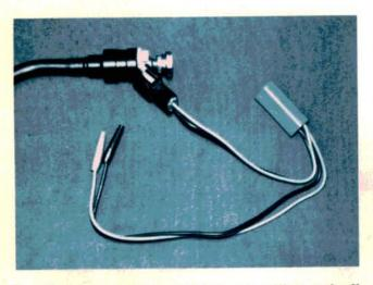
In order to measure K-Lambda duty cycle with your dwell meter, use an adapter harness such as this Thexton item (P/N 391) to connect the meter to the frequency valve. Put the meter on the 90-degree scale. To convert duty to dwell, multiply duty cycle times 90 percent.
