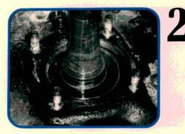
Raise the vehicle and remove the rear wheels and brake drums. Remove the brake lines. Remove the bolts that hold the bearing retainer on the axle housing. Disconnect the brake cables using one of the methods mentioned in our introduction. Slide the axle assemblies out of the differential.
