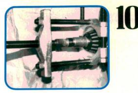
Now we're ready to pull that inner pinion bearing if it's bad. It's on there, believe me. You want a puller that gets under the inner race. A puller that grips the bearing cage may simply disassemble the bearing and leave the inner race on the pinion shaft. Bummer.
