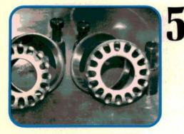
Remove the bearing caps, adjusting collars, and bearing races. Match them as sets in two separate piles. We want the races and bearings to go back together as matched sets if we plan to reuse the carrier bearings. Inspect the bearings and races as usual and replace as necessary.
