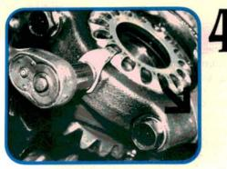
Remove the differential carrier and unbolt the lockplates that hold the carrier bearing adjustment collars. Match the bearing retainer caps and the bearing cradles with sharp punch marks. That way you'll be sure to get them back together as a matched set. Don't laugh, it's easy to get them confused.
