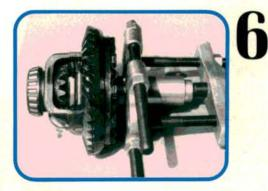
Use a setup similar to the one shown to remove the carrier bearings. Make sure the puller grabs the inside race, not just the cage. When you press or drive the new bearings back on the assembly make sure the press tool bears only on the inner race or you'll ruin the new bearing installing it.
