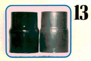
The crush spacer at left is the old one. If you look closely, you'll notice that it's slightly shorter than the new one at right. It's already been compressed once. Never reuse the old one. That's asking for trouble. We have to properly preload the inner races to make the bearings last.
