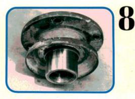
Take the companion flange and inspect the sealing surface for any nicks, cuts or gouges that might ruin the new pinion seal. Minor imperfections, or nasty accumulations of surface rust and dirt can be removed with fine emery. Replacing the pinion seal without this step is a waste of time.
