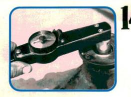
Install the front pinion bearing, slinger, and pinion seal. Push the pinion through the bearing and flange. Torque the pinion nut to an initial torque of 110 Nm (80 ft-lb). Turn the flange several times. Check initial turning torque. Slowly tighten the nut to get proper turning torque.
