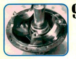
Thoroughly clean the differential carrier housing. Inspect the bores into which the pinion bearing races fit. Make sure you didn't raise any burrs with the punch when you drove the old races out. If you're replacing bearings, the old races make great drivers. Safety glasses, please.
