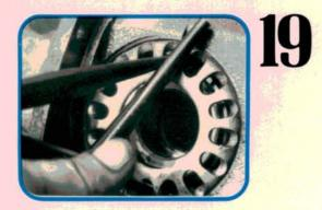
If you don't have the proper tool, you can turn the collars with punches as we did. Adjust the collars for zero bearing clearance, then alternately screw one collar out and the other collar in—in equal amounts—to get the correct backlash. In this case it's 0.13-0.18 mm (0.005-0.007 in).
