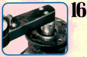
Believe me, this is important. We just can't leave the pinion bearings too loose. At the same time, we have to strike a delicate balance between too loose and way, way too tight. Tighten to get proper preload without exceeding the maximum torque for the pinion nut of 234 Nm (173 ft-lb).
