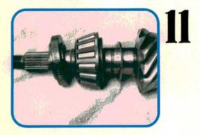
When replacing the old with the new, don't forget the pinion depth adjusting shim or there'll be big trouble in River City. A spacer like this one from Miller has a collar that rides on the inner bearing race but misses the cage. Do not press on the cage of the bearing or you'll trash it.
