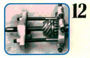
Reinstalling the pinion bearing was just a matter of using that shouldered spacer we just mentioned and the same gear puller. Only this time we used the pinion as our leverage point and used the puller to pull the bearing over the pinion shaft. It's just a matter of leverage.
