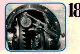
Mount a dial indicator as shown. Make sure the dial indicator is at a right angle to the ring gear tooth being measured. Preload the gauge and zero the dial. Hold the pinion so it can't turn and rock the ring gear back and forth against the pinion, measuring total gauge travel.
