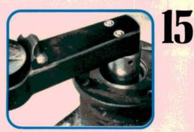
You have to keep checking initial turning torque each time you tighten the pinion nut. New bearing 1.17-1.87 Nm (10.9-16.5 in-lb). Old bearing 0.56-8.7 Nm (5.2-8.7 in-lb). This is the force needed to get the bearing moving. This is the amount of torque needed to get the shaft STARTED turning. Never mind what it reads AFTER it's turning. This is preload.
