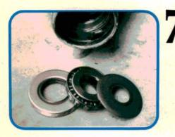
Use a soft mallet to drive the pinion through the front bearing. Remove the pinion seal, oil slinger, and the front pinion bearing. Clean the bore where the new seal will ride. A thin film of sealer on the outside of the seal will help seal any small imperfections in the bore caused by rust.
