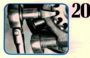
Tighten the collar away from the ring gear 1 to 1<sup>1</sup>/<sub>2</sub> notches to preload the bearings. Recheck backlash. Install the lock clips. Tighten the bearing cap bolts to 69-88 Nm (51-65 ft-lb). Add 3.5-5.2 in-lb to the initial preload spec and check total preload (turning torque) of the ring and pinion.
