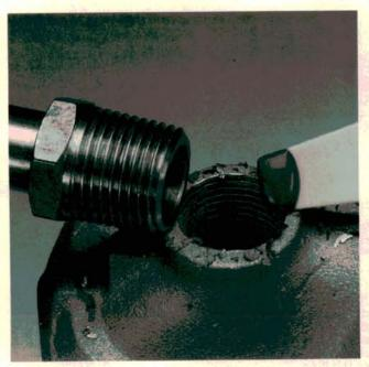
This thread-forming chemical is anaerobic—it sets up in the absence of air. If any excess chemical oozes out of the stripped hole, just wipe it away. The chemical creates reusable threads that will not corrode.
