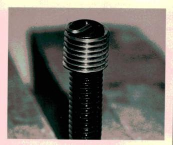
The typical coiled insert installing tool has a little notch that grabs the tang on the insert. Some kits have metal tools, others have plastic. I prefer metal tools because I've seen the notch peel off the plastic ones.
