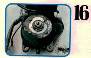
That corrosion buildup on the outside was only the tip of the iceberg. Beneath the cover, we found this barnacled driven hub. We had to "unearth" the four screws holding the drive hub to the gear drive. Fortunately, a new hub and screws are provided with the replacement mast.
