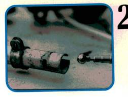
Insert the new mast in the guide tube and fully extend it. Guide the remaining nylon cable through the small hole in the neck of the plastic housing and reinstall the guide tube on the plastic housing. Apply silicone sealer where they join. Don't forget the screw/clamp and ground wire.
