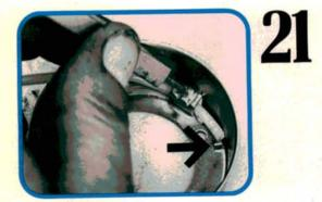
Install the nylon cable in the new driven hub. You don't have to keep track of which way the cable goes. Just use the raised tab as a stop for the cable. Place the hub on a hard, flat surface. Take a punch and stake the cable retainer tab down against the cable, just enough to hold it tight.
