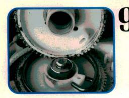
Try to turn the top gear while holding the lower one. There should be a springing action between the two, but you shouldn't be able to turn one without the other turning too. If that does happen, remove the circlip and top gear. Check that neither of the ears that sit in the clutch spring are broken.
