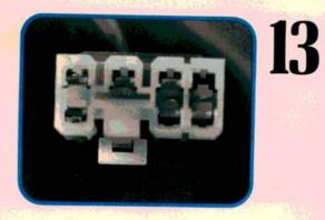
Wire values at the multipoint connector are as follows: With the key in the on position, and the radio on, all wires except the white and black ground wire are hot. Key on, radio off? The yellow, white/blue, and red/green wires are hot. Key off? Only the white/blue wire is hot.
