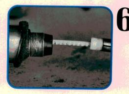
Now finish unscrewing the collar holding the mast to the guide tube and pull the mast (or whatever is left of it) and the toothed cable from the assembly. Check the guide tube for signs of corrosion or damage. Clean and lubricate as necessary before reinstalling the new mast.
