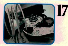
To save time, just snip the old nylon drive cable and discard it along with the old drive hub. There's no sense trying to free the cable from that old rusted hub. The Toyota, unlike the BMW, does not have a toothed cable. Its nylon cable is held on the drive hub by a single crimped tab.
