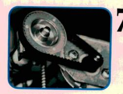
This ribbed belt runs between the drive motor and the worm gear. We checked to see if any of these internal parts were available, and they weren't. So please handle these internal components with care and make sure everything is clean and turning freely before you reassemble the unit.
