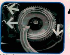
With the cover removed, we can see the drive mechanism. Remove the crescent-shaped, plastic retainer to expose the toothed drive cable and rollertensioner that keeps it tight against the drive gear. Remove the two screws at left that hold the motor in place and pull it off to the side.
