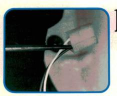
Before condemning an inoperative antenna on this BMW, check to see it's getting power. With the ignition off, the red wire should be hot. Key on? Both wires should be hot. This takes a second to check and saves the embarrassment of removing and disassembling the antenna for a dead wire. Also check the ground connection to the chassis.
