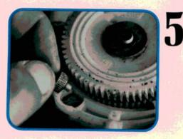
Now remove the small metal roller-tensioner. Note that the drive gear has an upper section that's driven by the motor, and a lower section that drives the toothed cable. With the roller removed and the drive motor off to the side, the drive gear will rotate freely.
