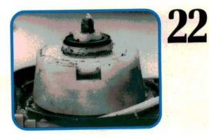
Before we reinstall the driven hub, we'll have to slide this drive gear back on the shaft. See the small notch on the drive? The retainer tab we just staked over the cable fits in this notch when we put the driven hub/cable back on. Leave the antenna mast fully extended. Reinstall the four screws on the hub.
