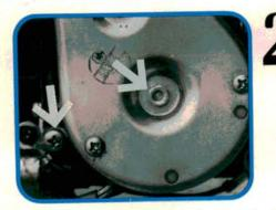
Reinstall the cover—two bolts and the lower support bracket—the phillips screw (arrow) and the small nut on the gear shaft. Now just lay the fully extended mast in the trunk and operate the drive motor to wind the cable. Reinstall the antenna.
