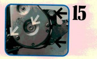
Remove the center nut on the cable drive cover, the two bolts holding the lower support bracket, and the phillips screw at left. You don't have to remove the other two phillips screws on the cover to do a mast replacement. Remove the cover. Note the location of any washers on the shaft.
