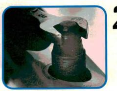
Carefully unscrew the trim collar (needle nose pliers worked well in the slotted collar). Then loosen the threaded collar below it that holds the mast in the guide tube. This is much easier than fighting corroded threads on a workbench. Now remove the assembly.
