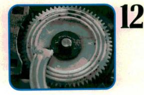
Reinstall the motor screws, the crescent shaped cable retainer, and the motor housing cover. Now plug in the motor, ground the ground wire with a jumper, and let the motor wind in the cable. Reinstall the antenna making sure the mount bracket is properly grounded, and you're all done.
