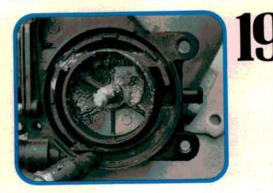
Lift the drive gear off the shaft. We're down to the motor and worm drive, and the bare plastic housing. Wash away that dirt and rust and blow the housing dry with compressed air. Make sure the hole in the neck of the housing for the new cable is clean and lubed. Relube the worm drive and shaft.
