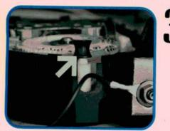
Remove the plastic cover from the assembly by carefully prying back on the plastic snap clips that hold it in place. Don't lose the rubber bumpers between the housing and the cover. This is important as the drive mechanism "floats" between the housing and cover on six of these. Check the ground connection to be sure it's clean and tight.
