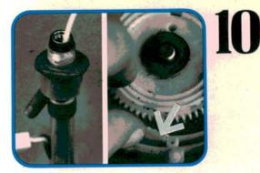
Slide the new drive cable down the guide tube and route it around the lower drive gear and into the opening in the storage reel below the gears. Line up the drive teeth on the cable with the drive teeth of the gear. Reinstall the roller tensioner to keep the cable tight against the gear.
