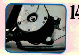
The antenna in the Toyota just growled but wouldn't go up. When we removed it we noticed a heavy buildup of rust around the mounting bracket. We also noted that kinked drain tube, its opening plugged with a huge wad of rustproofing. Not good signs. A clean, unkinked drain is essential.
