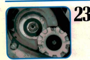
Take the time to thoroughly clean away all rust and corrosion from the inside of the drive assembly cover. We don't want the driven hub rubbing or binding in here. Also be sure you didn't lose that small washer between the cover and the driven hub. Make sure there's some lube between the two.
