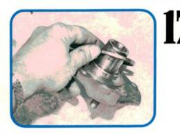
The bearing's gone. Remove that old seal and discard it. Thoroughly clean the sealing lip where it rides. Check the hub shaft where it presses into the bearings for pits or rust. Unbolt the old rotor and remove it. Remove any rust or dirt that could keep the new rotor from sitting squarely on the hub.
