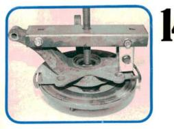
Rather than use a slide hammer, we made this portapress to free the drive hub in this GLC. The press bar bolts on at the hole for the ball joint pinch bolt and the lower hole for the strut-to-knuckle attaching bolt. We used an old VW valve adjusting shim between the screw and the drive hub.
