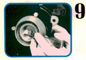
If you had too little end play, or none at all, the spacer is too thin. You can get a close idea how much thicker the spacer needs to be by holding the bearings in their races as shown and checking the gap between the inner races and the spacer. It's either that or start substituting thicker shims at random.
