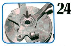
When the Mazda hub is fully seated, the inner face of the hub will ride at the lower edge of the chamfer on the inner bearing race (arrow). Take a moment to be sure the hub turns freely in the bearings. Install the inner grease seal. Reinstall the disc brake caliper frame.
