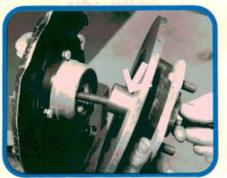
Install the rotor on the drive hub, making sure the locating surfaces between the two are clean. Alternately tighten the bolts that hold the rotor to the hub to their proper torque. Make sure the shaft on the drive hub is smooth and free from rust (arrow) and apply a thin coat of grease to it.
