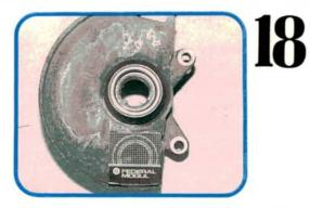
Drive out the old races like you would on a spindle type front end. Clean the bores for the races and check for nicks or gouges. Drive in the new races. Pack the new bearings with grease and install them with the original spacer between them. Install the new seal on the drive hub side of the knuckle.
