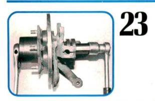
We used the on-the-car wheel bearing press from Schley Products to press the drive hub/rotor back into the bearings. Set the tool to press on the head of the drive hub at one end, and the inner race of the inner bearing on the other. Then just tighten the big screw and pull them together.
