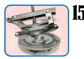
Looks like the Nissan doesn't it? Don't make the mistake of just leaving the bearing and outer seal on the drive hub and pressing them back in place. The seal will cock and jam in the knuckle and simply won't seal as it should. You'll end up with grease on the pads and water in the bearings.
