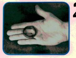
Remove the drive hub and clean away the excess grease. Then retrieve this spacer. This little devil sits between the inner races almost like the crush spacer between pinion bearings. Most of the time, if you're only replacing bearings, end play won't change. End play should always be checked, however.
