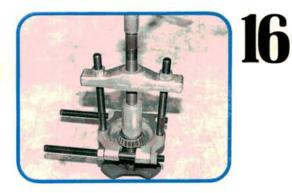
Here's another puller you might try using to pull the bearing from the hub. It's the same one from Miller Special Tools we used on the Toyota ring and pinion job in the September issue. It fit between the bearing and seal and pulled against the inner race, removing the bearing without damage to it or to us.
