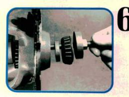
Once again. Make sure everything is clean. This is a close tolerance and it won't take much to throw things off. Insert the tool through the bearings and the original spacer. Tighten slowly, keeping the spacer centered between the inner races. Seat the bearings with a torque of about 6-13 Nm (5-10 ft-lb).
