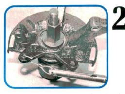
The factory suggests this method for checking bearing preload. Bearings and spacer are in place and the bearings loaded. Attach a spring scale as shown and measure how much force it takes to get the drive hub turning from a dead stop. Always compare readings to the specifications for your car.
