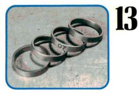
If your shop does a lot of this work, it may be worthwhile to stock a selection of these spacers. These checks will be especially important when you replace a collision damaged knuckle. You just can't take the chance that you'll get lucky enough to get a replacement knuckle that uses the same spacer.
