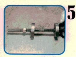
Make a special tool like this one from a length of  $\frac{1}{2}$  inch rod. You'll need two large washers or discs like the ones shown. The discs have to be just large enough to bear on the inner bearing races. This tool will simulate what happens when the drive axle is inserted through the hub and the nut is tightened.
