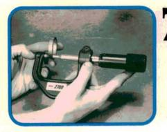
With the tool installed and tightened, mount a dial indicator as shown. Rotate the hub to make sure the bearings are fully seated. Then take your reading. You should have 0.01-0.05 mm (0.0005-0.002 in) of end play. If you're right on the money you'll have a reading of 0.025 mm (0.001 in).
