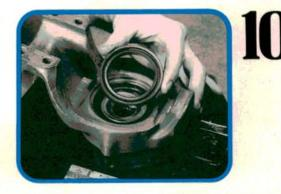
Once you've selected the proper spacer, pack the bearings with the recommended grease. Install the bearings, spacer, and the outer grease seal. Always use new seals. Check the sealing band on the outboard drive joint where it rides in this inner seal for rust or pitting that could cut the seal.
