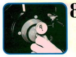
If end play is greater than specifications, the spacer is too thick. Subtract allowable end play from your dial indicator reading. This is how much thinner the spacer needs to be. Write this number down. Mic the original spacer and subtract this number. Select a spacer of that thickness.
