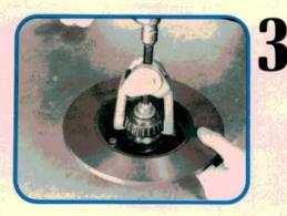
The outer bearing will always stay firmly attached to the drive hub. The outer seal is below it. Use a puller or press tool with fingers long enough to grip between the inner race of the bearing and the drive hub shaft. If you grab the cage, you'll ruin the bearing for sure, and it could fly apart.
