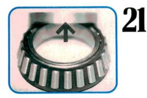
Changing spacer thickness changes the preload on the bearings. Mazda numbers their spacers, with each number corresponding to a specific thickness. A change of one number changes spacer thickness by 0.04 mm (0.0016 in) and changes preload by 0.2-0.4 Nm (1.7-3.5 in-lb).
