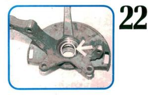
If preload is too great, the shim is too thin. If preload is too light, the spacer is too thick. Figure how much thicker or thinner the shim has to be. Then remove the threaded tool and inner bearing. Install the correct shim. Reinstall the inner bearing and tool and double check preload.
