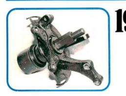
Mazda's repair manual says to tighten the threaded bearing loader in steps of 50 Nm (36 ft-lb) to a final torque of 200 Nm (145 ft-lb), checking as you go to make sure the bearings aren't binding. You'd need a heavier threaded tool like this on-the-car bearing installer from Schley Products.
