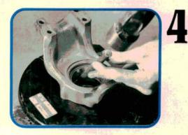
If you're replacing bearings, take a punch as shown and drive out the old races. Throw the bare knuckle in the cleaning tank to remove any crud that could keep the new bearings from seating properly in their bores. If you did raise any metal with the punch, carefully file or sand it smooth.
