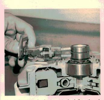
The apply current for the magnetic clutch flows through these brushes and slip rings on the rear side of the clutch assembly. The brushes, which are serviceable, are sealed to protect them against dirt and moisture. The ECVT computer regulates current flow through the clutch.
