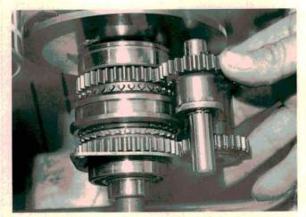
To change directions, the ECVT uses this simple, fully synchronized gear set and hub assembly. On the output side of the drivetrain, the Justy ECVT has a conventional spider gear-equipped differential setup. It also has a set of reduction gears.
