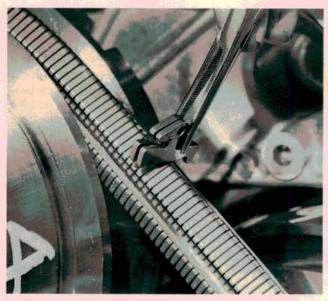
Here are two of the 280 or so steel segments that make up the Van Doorne drive belt. As you can see, it's really more of a loop than it is a "belt." In a giant and constant domino effect, each little steel segment pushes the segment ahead of it. This belt transmits power by pushing instead of pulling.
