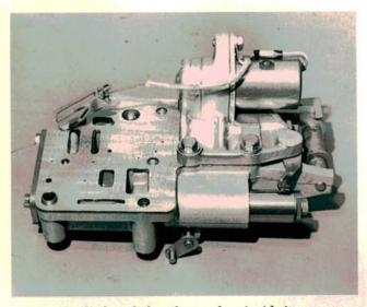
ECVT valve body only has three valves inside it: a pressure regulator valve, a shift control valve, and an engine braking valve. The three-way solenoid on the valve body reduces pulley clamping pressure during light throttle cruising.
