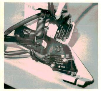
This pair of simple on-off switches mounted on the gas pedal assembly gives the ECVT computer its throttle position signals. Because these switches mount in fixed positions, you don't even have to adjust them when you replace them.
