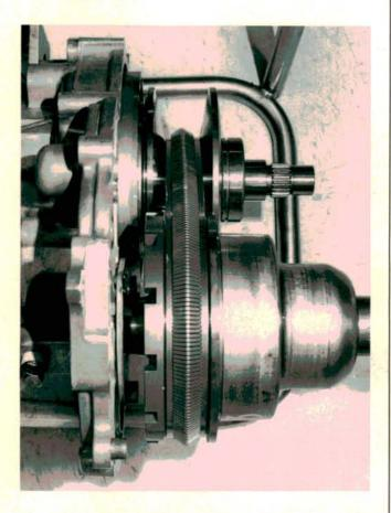
The drive pulley is in the background, the driven is in the foreground. The ECVT will use a basic Dexron-type fluid. You only need a handful of special tools to tear down and reassemble the entire unit.
