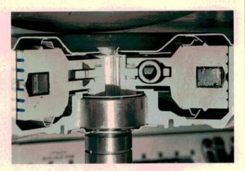
In this cutaway of the magnetic clutch assembly, you can see the magnetic coil's wire strands in the center of the rotor unit. When the clutch engages, the stainless steel powder in the rotor grooves (highlighted in blue) locks the rotor to the drum. Subaru engineers say this unit will be sealed and non-serviceable.
