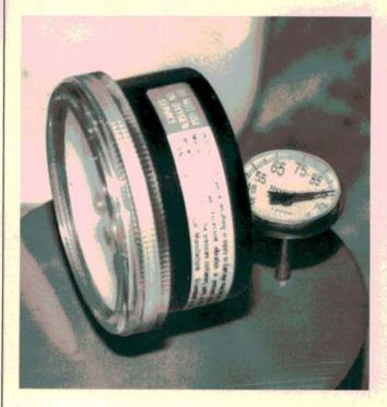
Let the assembly sit for two minutes. Then hold the assembly firmly, tilt it downward at about a 45 degree angle and shake it with enthusiasm. Turn the assembly upright and write down the gauge reading and the temperature of the water. Compare the readings to the chart in the kit to calculate Reid vapor pressure.
