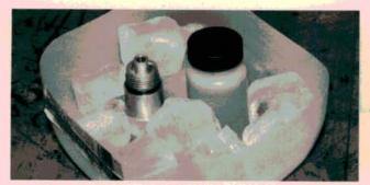
Take a fuel sample. Chill it and the fuel cup and holder. We're going to chill the fuel, then warm it and measure the pressure it gives off as it vaporizes. Certain fuel additives can make the fuel vaporize at lower temperatures. Fuel percolation or vapor lock can cause all sorts of problems.
