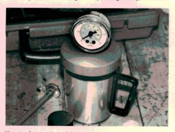
Here's a better view of the assembly. Here, we're warming the chamber. Later, we'll screw the chilled fuel holder into it. The thermometer at the left is inserted in the lid just behind the pressure gauge. Water temperature will be an important part of our final calculations.
