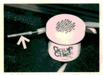
To check for water, coat the metal tip in the wand with paste, draw it into the plastic sheath. Then insert it through the filler neck until the tip reaches the lowest part of the tank. Withdraw the wand and inspect the paste on the metal tip. Water will make the paste change color—from green to red. Miller Special Tools has a kit available that allows you to make some very important tests to find out if the car is burning good gas or some contaminated chemical catastrophy.
