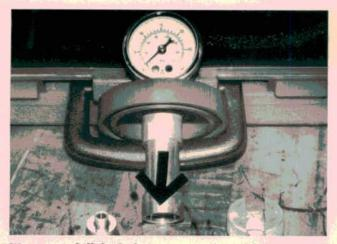
We want to chill the fuel. But we want to warm the pressure tester. Fill the thermal cup to within ¾ inch of the top with warm water of 43.3 degrees C (110 degrees F). Place the fuel chamber (arrow) in the water to warm it. If the temperature drops below 40.6 degrees C (105 degrees F), reheat it.
