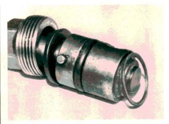
If your engine is as carboned as this, you may have to fabricate a small hook and dig for this copper seal that goes between the auxiliary valve and the combustion prechamber. An old bicycle spoke with a small hook on the end will work. Always replace the seal with a new one.
