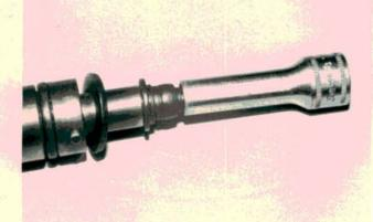
Remove the old seal with a pair of pliers. We found that a deep-well socket worked nicely as a seal installation tool. Don't loose the lower spring seat while the seal is off. If the seat and spring washer do fall off on the bench, the spring washer is marked with the word "up."
