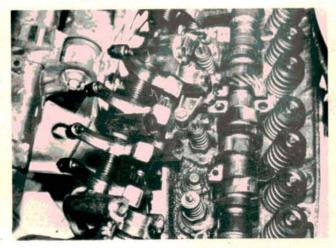
Remove the rocker shaft assembly and lay it aside. Unscrew the valve holder from the cylinder head and remove the valve assembly. Pull the valve chamber now and install new crush-style sealing washers or you may have a compression leak later.
