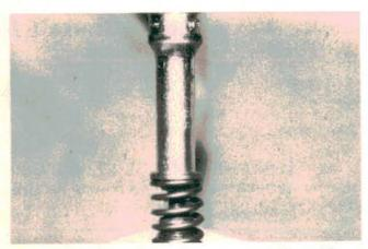
You can hunt for a valve spring compressor if you like or you can just put a socket over the valve spring retainer and rap it with a small mallet. The impact will break any carbon loose, and will usually cause the valve keepers to pop free. Remove the retainer and spring to expose the seal.
