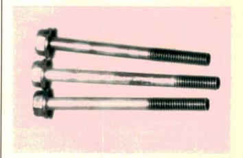
Clean the mating surfaces between the rocker assembly caps and the head. Put a small amount of non-hardening sealer on the mating surfaces of the end caps. Reinstall the rockers. The three bolts front and center on the rocker assembly are not the same length. The long one goes in the center hole.
