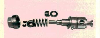
Here is an exploded view of the valve assembly. Always replace that o-ring on the valve holder. Clean the valve itself with a wire brush. Check the valve and valve holder sealing faces. Also check the valve stem where it rides in the seal for any roughness that could cut or ruin the new seal.
