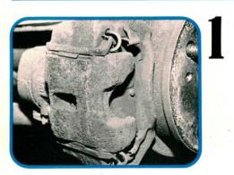
Take a good look at the calipers and rotors before you start to take anything apart. Any sign of fluid leakage? Standard rotor thickness is 10.0 mm (0.39 in) and replacement thickness is 9.0 mm (0.35 in). There isn't much meat on these rotors for resurfacing so measure carefully before quoting the job.
