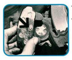
The rear brake pads have a small protrusion on their backing plates. The caliper piston notches must be in the 9 and 3 o'clock position to properly engage the pad. A little silicone spray on the piston dust boot will keep it from hanging up on the piston as you index it.
