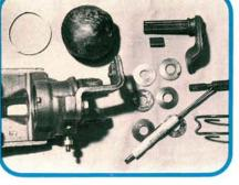
Before reassembling the caliper, examine all internal parts carefully for any damage, wear, or corrosion. The spring washers must be installed on the adjusting bolt with their faces in an alternating convex, concave order. Start with a convex face against the adjusting
