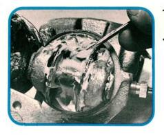
With the boot cover out of the way, inspect the parking brake assembly for water damage. Any brake fluid leakage from the adjusting bolt o-ring would show up back here too. Clean the old grease off of the mechanism. There should be a small roll pin installed next to the torsion spring.
