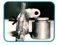
Remove the parking brake crank snap ring. The tool must straddle the parking brake and push down on the stack of spring washers below it. There isn't much pressure involved here but you may have trouble getting the tool positioned right. Catch the small part called the strut as the crank is removed.
