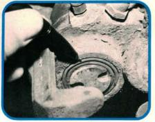
You don't have to wait until a caliper starts to leak before recommending an overhaul. If the dust boot or any of the other rubber parts is torn, dried out, or just generally tired looking; trouble isn't too far behind. Check for smooth operation of the parking brake
