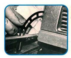
Remove the screws bordering the glove box insert. The glove box has to be removed so you can disconnect the right side defroster ducts from their support brackets beneath the dash and from the blower housing. Remove both the left and right under-dash panels, held by plastic fastener clips.
