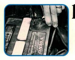
Once you've made sure everything works in the dash (lights, radio, and so on), disconnect the battery negative terminal before disassembling the dash. You don't want to add a wiring harness to the parts list! This particular car needed to have battery posts and terminals cleaned anyhow at 116,000 miles.
