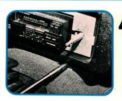
Remove the side panels from the console. When you remove the screws holding the console trim face from the console support brackets, don't forget the two screws hiding just below the radio. If you forget them, you may crack the plastic. We've also removed the face plate holding the radio in the console.
