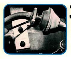
With the glove box removed, we can see the support brackets for the defroster ducts. Remove this retaining clip at the vacuum pod and the vacuum line. Then push the rubber mounting tabs through the metal bracket to free the duct. Let the vacuum pod hang from the duct, but don't remove it.
