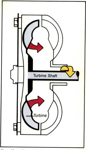
If we add a turbine attached to a turbine shaft, it will turn as the fluid from the pump strikes its blades. This causes the turbine shaft to turn, transmitting force to the transmission.
