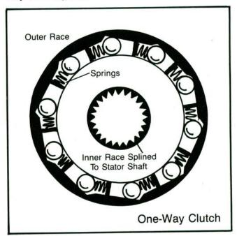
The stator has to resist the difference in fluid force between the pump and turbine until those forces equalize. In one direction, the rollers jam tightly in their tapers locking the races. In the other direction, they freewheel, disengaging the races.
