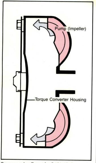
Our pump, or impeller, catches fluid inside the converter housing and flings it in the direction shown. The combination of centrifugal force and the shape of the fan blades sends the fluid spinning.
