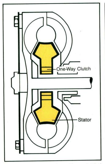
The stator sits between the two fans, making sure that fluid is directed back to the pump at the proper angle so it will work with the pump instead of against it.
