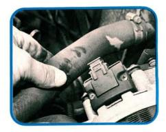
Start the engine. Double check to be sure the heater valve is open. Keep the system topped-off at the remote filler neck as any trapped air escapes. Gently squeeze and release the top radiator hose to help purge any remaining bubbles. The top hose should warm as the thermostat opens.
