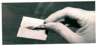
Shake the paint bottle, then apply a light first coat. Let the paint dry for at least a minute or until it's tack free. Apply the paint a total of three times, more if it's a really bad break. Clean the brush with lacquer thinner if you plan to use it again.
