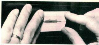
The paint should overlap the break by about one-half inch on either side. Wait twenty minutes after the last application, then carefully remove the stencil. Move the stencil to the next break and repeat the procedure.
