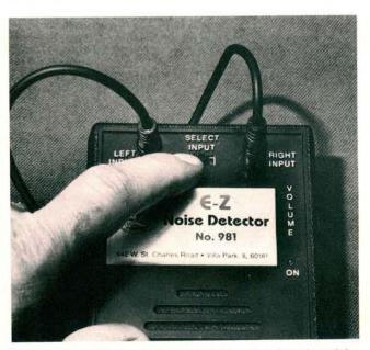
To compare noise levels from the left and right sides of the vehicle, simply flip this input selector button. There's no need to stop the car and move the clamp from side to side. The kit includes two extension cords for those noises at the far end of the car.
