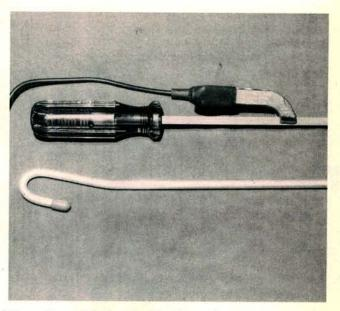
If you do need to look inside the engine compartment for the cause of a noisy alternator or water pump bearing, or need to locate the source of an engine noise, simply attach the probe included in the kit. Or use that long screwdriver for hard to reach places. You still have to be careful, but at least your head is safely out of the way.
