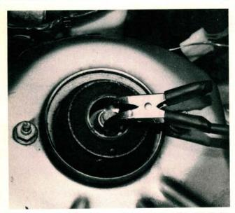
Here's an example of how you might use the E-Z Noise Detector. Place a clamp on each strut rod of a MacPherson strut suspension. Connect the left clamp lead to the left channel of the amplifier, the right clamp to the right channel. Noises from the brakes, drive joints, or wheel bearings will travel up the rod.
