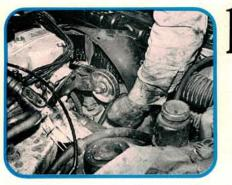
Since this engine has been used in so many different cars, we'll discuss the initial steps of the job only in general terms. No matter what you're working on, you'll need to make room for yourself at the front of the engine. Disconnect the battery and drain the cooling system. Remove the fan, fan shroud, and radiator.
