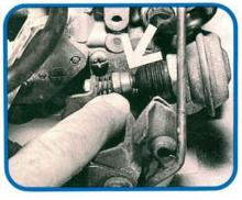
The carburetor dashpot (arrow) provides a cushion when the throttle is closed rapidly. This allows a more gradual transition between the leaner air-fuel ratios of cruising and the richer idle ratios. If the dashpot touch speed is too low, it may cause stalling during fast stops or deceleration.
