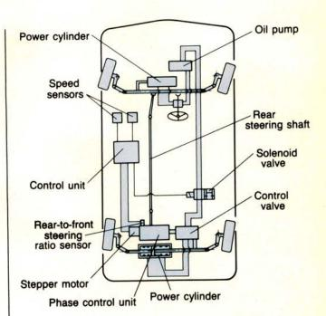
The real heart of this system is called the Phase Control Unit. Decisions made by the Control Unit are translated into movement of the rear wheels by this unit. Once you understand how the Phase Control Unit functions, the rest is easy. The phase in Phase Control refers to the front and rear wheels' relationship to one another. Front and rear wheels turning in the same direction are said to be in the same phase, and opposite phase if they are turning opposite one another.
