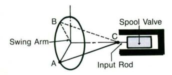
Moved By Bevel Gear (Steering Wheel Turned Left)
