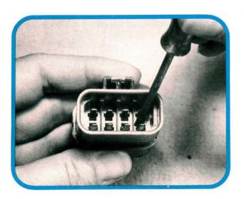
Removing the terminals from the carburetor connector makes it much easier to remove individual components during disassembly. Remove the black plastic retainer from the back of the connector. Pry gently on the plastic latches inside the connector to release each terminal. Note terminal locations for reinstallation.
