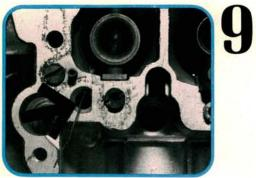
Slide a thin piece of copper wire (arrow) through the accelerator pump discharge port. Dirt has a nasty habit of blocking this passage. Remove the primary and secondary air bleed jets and clean their passages. The panhead screws cover smaller passages for the Enrich-
