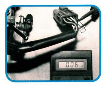
Check the operation of the Throttle Switch with an ohmmeter. Back-probe the carburetor connector with two paper clips. Work the throttle shaft open and closed several times by hand. The Throttle Switch should make and break continuity cleanly. Check for sticking switch contacts.
