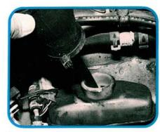
Here's a maintenance item you might be overlooking. Subaru recommends changing the brake fluid at 15,000 mile intervals. Siphon the old fluid out of the reservoir, then refill with fresh fluid. Proper bleeding sequence for this dual-diagonal system is left rear, right front, right rear, then left front.
