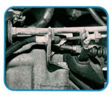
The PHV is linked by cable to the clutch linkage. Check for proper PHV cable adjustment during brake service or when the clutch cable is adjusted. The brakes should release just as the clutch begins to take hold. Hold the cable with pliers to keep it from turning during adjustments.
