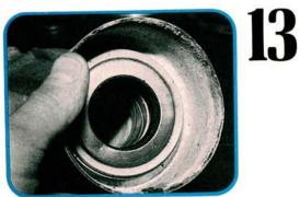
An out of balance or damaged driveshaft may have caused excessive extension housing bushing wear. Inspect the driveshaft yolk for roughness or seal grooving. Maximum bushing wear limit is 38.075 mm. Replace the extension housing seal and polish minor abrasions on the driveshaft before reinstallation.
