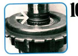
The hollow sun gear shaft is backed out so that you can see where the seal rings fit. Oil passes through this opening (arrow) to lubricate the rear one-way clutch. Check the inside surface of the one-way clutch assembly for wear. The A43 uses larger diameter sealing rings.
