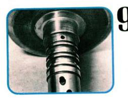
Inspect the area around the governor seal lands for bushing wear. The governor passages must be clean and free of any debris. The governor clips to the output shaft and covers the two large passages. Disassemble and clean the governor; they've been known to stick.
