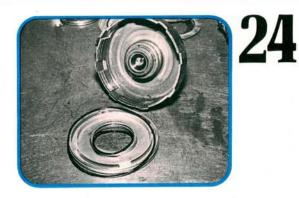
The outer o-ring seal cross section, clutch piston groove diameter, and clutch piston groove width on both the forward (shown) and direct clutches were changed in August 1981. The earlier, smaller o-rings will not seal properly on the later A41. Later, wider o-rings will bind the clutch piston if used on an A40.
