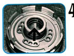
The bushings on the inside of the center support (arrow) are the most prone to wear. The bushings support the end of the sun gear shaft and handle the input torque from the forward and direct clutch units. Wear limit for the bushings is 36.461 mm. Inspect the sun gear mating surface also.
