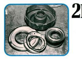
The direct clutch is a two piston design. During third gear operation, torque demands are low and only one piston receives hydraulic pressure. When reverse gear is engaged, a sequencer valve in the valve body applies both pistons for increased holding power in this hightorque situation.
