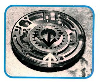
Inspect the oil pump torque converter bushing. Engine-to-transmission misalignment or excessive flexplate runout will cause increased bushing wear. Inspect the mating surface of the torque converter for seal or bushing wear. New bushing inside diameter is 38.113 to 38.138 mm. Wear limit is 38.188 mm.
