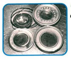
The low-reverse brake also has dual pistons. A sequencer valve in the valve body applies the two pistons one after the other, reducing shift shock when engaging reverse gear. The reverse brake outer piston is also applied in park. Assemble all three piston parts before reinstalling them in the case.
