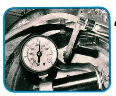
Hook your vacuum pump to the delay valve at the tee between the air intake door and the bleed valve. When intake air is cold (forget engine temperature), this circuit should hold vacuum to keep the vacuum door in the warm air intake setting. Cold, wet air can ice the carb even on a warm engine.
