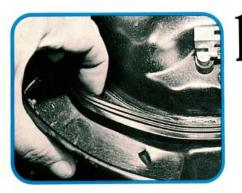
Several Honda technicians complained about replacement air filter cartridges that distort the rubber sealing rings in the air cleaner housing. If the replacement air filter has rubber sealing surfaces top and bottom, it may be too thick. The additional thickness distorts this seal and allows dirt to enter the carb throat.
