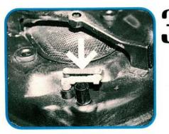
We removed the small protective cover on the air bypass valve in the air cleaner so you could see it better. This bi-metallic spring opens when intake air is warm, and vents vacuum away from the air intake door. The door then opens to outside air. A tiny vacuum leak like this also raises hot engine idle slightly.
