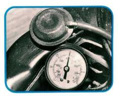
Check the air intake door control diaphragm to make sure it isn't ruptured. Even if it holds vacuum, check for smooth movement of the door itself. Make sure it moves from fully open to fully closed with no unscheduled stops in between. A bad intake door can result in cold hesitation or carburetor icing.
