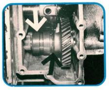
Use angle-tipped snap ring pliers to move this snap ring (black arrow) out of its groove. Then slide it to the end of the input gear. Now push the collar (white arrow) that splines the input gear to the cluster gear away from the cluster gear. Angle the gear and collar through the opening in the case.
