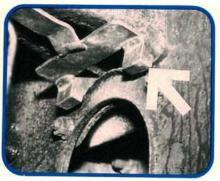
Engine and transaxle removal could be an article all by itself. If you're a first timer, consult a service manual for more detailed information. Remove the right front wheel; then raise the lower control arm with a jack. Placing this tool (arrow) under the upper control arm unloads the lower ball joint.
