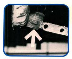
Remove the boot clamps from both inner CV joints and slide the boots back. Remove the two bolts holding the right lower ball joint (arrow) to the control arm. Push the right spindle and hub assembly outward until the right tripod joint clears the inner CV joint. Prop the ball joint in this position.
