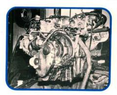
Install a spring retaining tool in the pressure plate before disconnecting the clutch hydraulics. Consult a manual for the specific parts that must be removed before the engine and transaxle can be removed. This was a 900 Turbo so there were extra parts to remove before they were hanging high.
