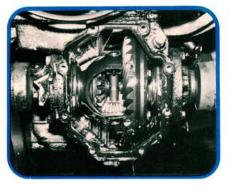
Remove the differential cover. Remove the bolts from both differential side bearing carriers. Remove the left carrier carefully to avoid damaging the plastic speedometer gears. The shims between the carriers and the case adjust side bearing preload and backlash. Keep each shim with its proper seat.
