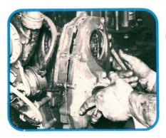
If you don't want to wrestle with the transaxle on a bench, leave it attached to the engine. Refer to the "Saab Clutch Replacement" article in the February 1989 issue of Import Service for details on 900 clutch removal and replacement. Start by removing the primary gear case front cover.
