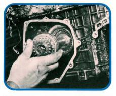
Remove fourth gear and its synchronizer assembly. Remove the three-four selector shaft. Take out the three-four synchronizer hub, sleeve, and selector fork. Inspect the sides of the selector fork for wear in the area where it rides on the synchronizer sleeve.
