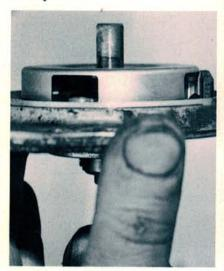
Remove the distributor cap and check for interference between one of the trigger windows and the pickup. The distributor rotors on these cars are very hard to remove, and someone may have tried to pry it off, bending the trigger window. This interference can cause a miss. It also throws up very fine, hairlike metal shavings that get magnetized and stick to the pickup.
