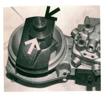
Position the jig on the mouth of the sensor cone, with the arrow on the jig facing the fuel distributor. Turn the adjusting screw until the magnet just touches the sensor plate. Then lift the larger, knurled collar to its first stop. The sensor plate is now positioned to do an APS adjustment.
