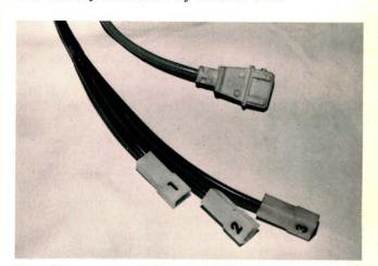
If you do any amount of work on KE systems, you should purchase the correct connectors and fabricate a patch harness, or simply buy one that's already made, like this Zelenda harness, P/N VW 1501. A harness saves a lot of time during hookups, and keeps you from damaging terminal ends.
