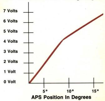
The Air Position Sensor is a potentiometer. It can travel a total of 18 degrees. The signal it generates is not linear, however. As you can see, the most rapid change in its signal occurs during the first 5 degrees of movement, when it's needed most.
