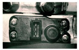
You saw this photo in an earlier article. To adjust the APS, loosen the four screws holding it to the fuel distributor. With the jig installed and raised to its first stop, rotate the APS and check for 0.2 to 0.3 volts. (Check between the center terminal and ground.) Retighten the screws and reseal them with RTV.
