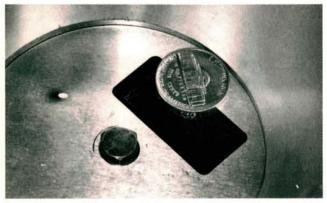
You also saw this photo before, but it's worth repeating. There has to be some free play between the sensor plate arm and the control plunger in the fuel distributor, up to a maximum of 2 mm. A nickel's worth is just fine, and when was the last time you accomplished anything with a nickel?
