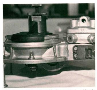
One other special tool that takes the guesswork and hassle out of APS adjustment is this adjusting jig, Zelenda P/N VW 1348/1A (formerly 134811). It has a magnet at its tip to grab and hold the air sensor plate, and preset detents that hold the sensor plate in the proper position for checking APS values at idle position.
