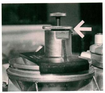
Make sure the jig fits flat and square. Lift it to its first stop. In this setting, the top of the sensor plate is even with the base of the cone. The jig can also be used to check injector fuel delivery rates at this first stop, or wide-open-throttle delivery rates when raised to its next, higher stop.
