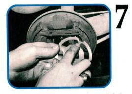
The rear suspension on this VW Rabbit presents a different problem. The stub axles bolt tight to the one piece axle beam, and no factory adjustment is provided. Now what? One possibility is to use a tapered full contact shim between the axle and axle beam to make the adjustment.
