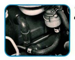
Most common service items are arranged for easy accessibility. The fuel filter is mounted below the carbon canister, on the right side of the firewall. The oil filter is mounted on the back side of the engine and can be reached from the top side of the engine.
