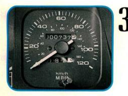
The Excel doesn't have any maintenance or oxygen sensor reminder lights to reset. It's up to you to remind the customer of his maintenance requirements. The oxygen sensor has a 50,000 mile replacement interval and the timing belt should be replaced at the 60,000 mile mark.
