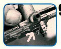
Occasionally, someone will overadjust things just a teeny bit. For whatever reason, if someone screws the needle valve seat down too far, the o-ring will pop through the opening on the bowl cover bore. Then, when they try to back it off, the o-ring catches and is torn and ruined in the process.
