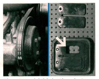
A loose air pump belt (left photo) keeps the air pump from delivering enough air to a three-way oxidizing converter. Manufacturers using pulsed air systems can also run into their share of problems. Pulsed air systems don't have the horsepower drain of an air pump, but damaged reed valves (right photo) in an air suction valve will allow exhaust gases to sneak back to the air cleaner, and reduce air flow to the converter at the same time.
