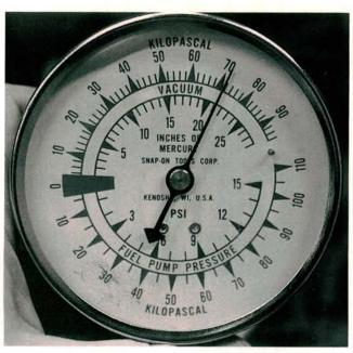
Here's a quick test for a converter restriction. Disconnect and plug the vacuum line to the EGR valve. Dig your trusty vacuum gauge out of your tool box and attach it to a manifold vacuum port. Rev the engine to 1500-2000 RPM. Vacuum should hold steady at 14-22 inches of mercury. Repeat the test at the same RPM with the brakes applied and the transmission in gear. If the vacuum reading drops steadily or the car stalls during either test, check for an exhaust or converter restriction.
