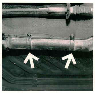
Since converters get hot, the addition of numerous heat shields have given new meaning to the word rattle. Shields like these on first generation Nissan Sentras and Pulsars are notorious for rusting loose and rattling. There's a pre-converter ahead of this pipe so it gets pretty hot too. The hose clamp, band aid approach is a popular fix, although welding or replacement of tattered shields is a better way to go. Resist the temptation to remove and discard any heat shield.
