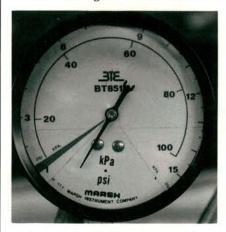
As a rule of thumb, most back pressure readings taken at the oxygen sensor port should run in the 0-3 PSI range. If you're getting readings way above that, it's safe to assume that there's a restriction in the exhaust system. You might have to do a little digging to make sure that the converter, and not another part of the exhaust system, is the source of your restriction.
