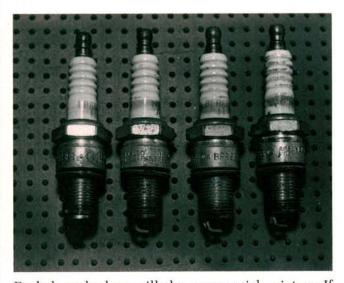
Fouled spark plugs will also cause a rich mixture. If the car has air injection to the converter, the extra air and unburned fuel give you everything you need for a first class afterburner. Fuel systems that are calibrated for very lean air-fuel ratios may cause a lean misfire at cruising speeds. The little bit of fuel available to the engine doesn't get burned as a result, and goes on down the pipe. The oxygen sensor may get a whiff of this unburned fuel and lean the mixture even further.
