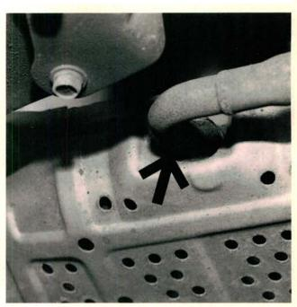
Three-way catalysts can only clean a controlled amount of pollutants. The rhodium in the three-way converter strips the oxygen from the  $NO_x$  emissions, leaving us with nitrogen and oxygen. For this to happen efficiently, the reduction of  $NO_x$  has to occur before extra air is pumped into the platinum and palladium bed by the air pump. The platinum/palladium bed needs the extra oxygen, since it's adding oxygen to make carbon dioxide and water.
