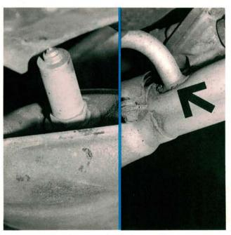
Some manufacturers keep reducing and oxidizing catalysts apart by installing two separate converters. The front (or pre) converter on this Subaru (left photo) contains a rhodium catalyst and does not receive direct auxiliary air. The rear converter handles HC and CO emissions, so an air induction hose (right photo) provides extra oxidizing air. Other cars use a single converter with separate beds. Only the oxidizing section gets fresh air.
