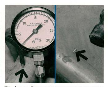
The absence of an oxygen sensor on some cars means you'll need a back pressure tester like this one from Forrest Manufacturing. Drill a hole in the exhaust ahead of the converter using the drill bit supplied with the tester. Insert the back pressure gauge adapter (left photo) and measure back pressure at that point. Drilling extra holes lets you locate the exact location of the restriction. After testing, install a self-locking plug (right photo) to reseal the exhaust.
