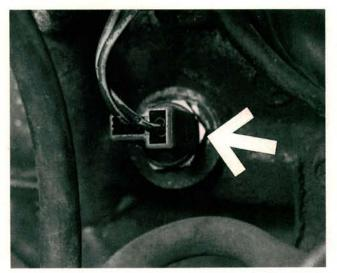
An inaccurate temperature sensor can fool the ECU into thinking the engine is still cold. The ECU will go on calling for a rich mixture from the fuel injection system, or carburetor, long after the engine has warmed up. A warm engine can't handle all the extra fuel and dumps the leftovers into the exhaust system. The catalytic converter isn't designed to handle the extra work load. Added heat caused by the rich mixture spells a slow death for the converter.
