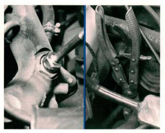
On vehicles equipped with an oxygen sensor, you can screw your exhaust back pressure gauge right into the threaded sensor hole. Remove the oxygen sensor and install the 18 mm test adapter (left photo). Don't overtighten the adapter or you'll strip some threads. This Borroughs gauge adapter uses the threaded end of an oxygen sensor. If the converter has air injection, block off the air supply (right photo) to the converter before beginning your test.
