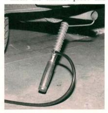
bring the engine and the analyzer up to operating temperature.
