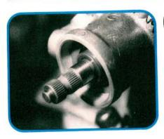
Take a close look at the pinion shaft. Don't go any further if it's scored or pitted in the seal area. Remove the rear housing Torx® bolts with an 8 mm 12 point socket. To remove the rear housing, hold the pinion assembly in place while turning and lifting the rear housing.
