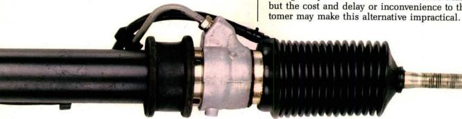
the boots and keeps them from collapsing or swelling when the rack is turned from side to side.
