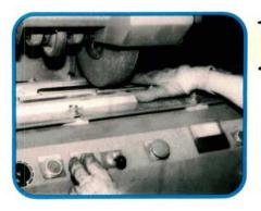
Don't try this at home kids. Rack remanufacturers straighten and polish Nissan rack shafts to remove small scratches during their remanufacturing process. This specialized equipment produces a finish that's as smooth as a new shaft. Special rack seals compensate for the difference in shaft O.D.
