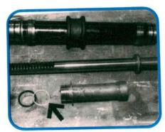
Remove the cylinder assembly (top), rack shaft (middle), and inner tube assembly (bottom), from the pinion housing. Separate the rack shaft from the cylinder assembly, then slide the inner tube off the rack. Discard the inner tube o-ring and set its nylon collar (arrow) aside.
