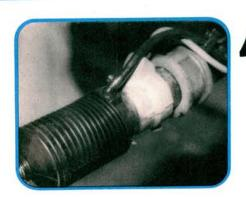
If the dust boots are full of fluid, you'll need to remove the rack whether you're rebuilding or replacing it. Prepare your customer for the worst before you start. Damage to other internal parts can make a rack overhaul either impossible or very expensive.
