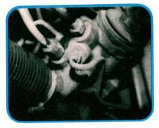
To pinpoint the source of an external leak, clean the rack thoroughly. Loosen, then tighten all line fittings to 20-26 Nm (14-20 ft-lb). Don't overdo it, the rear housing is only aluminum. Road test the car, then recheck for leaks. There's no sense removing the rack for an external leak.
