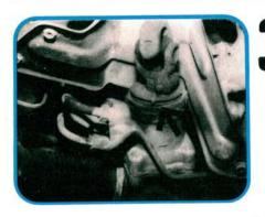
A difficult leak to fix, either on or off the car, is one coming from the pinion seal area (arrow). Leaks in this area are usually caused by a corrosion damaged pinion shaft. The roughness on the shaft damages the pinion seals. New pinion assemblies aren't available separately.
