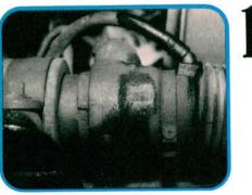
Start by determining where the fluid leak is coming from. A rack on your bench will have a hard time telling you where it was leaking. External leaks may be caused by loose or cracked fittings and lines, porosity or cracks in the steering gear housing, or a damaged pinion shaft seal.
