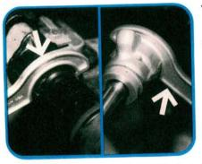
Loosen the pinion housing (left photo) and end housing (right photo) lock nuts with the special spanner (arrows). Rust can make it difficult to turn the lock nuts. You may need a small punch to get them turning. Remove the end housing and its bushing from the rack shaft.
