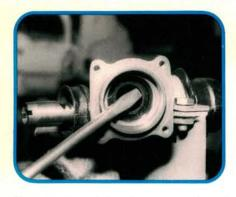
Remove the pinion housing oil seal with a large flatbladed screwdriver. Take the pinion housing out of the rack stand, then wash it in clean solvent along with the other disassembled parts. Remove and discard all o-rings, oil seals, and both lock plates. Dry all parts with compressed air.
