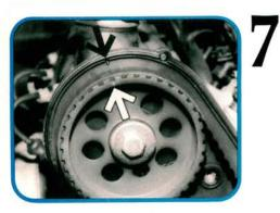
If you're not sure if you're on number one cylinder, look at these marks on the camshaft sprocket and inner cover. With the crankshaft "zeroed" these marks should align if you're on number one. If the belt has jumped a tooth, you'll have to remove the old belt and realign the camshaft.
