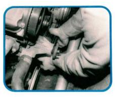
Remove the crankshaft pulley bolt. You should be able to remove the pulley by hand, but don't get rambunctious. Hold the pulley with both hands as shown and wiggle it slightly as you pull it off. The pulley is heavy and if it comes off too easily, a hard tug may send your knuckles crashing into the radiator.
