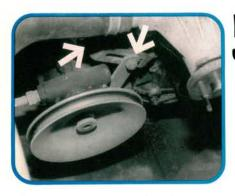
The screw tensioner for the power steering pump is directly below the water pump hose to the radiator. Loosen the pinch bolt in the support bracket (right arrow). Then back off the screw-jack tensioner bolt (left arrow) until you can remove the power steering belt.
