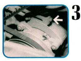
Here's one of those screw-jack adjusters used to tension the accessory belts. The alternator and power steering pump are held tight by one pinch bolt each, but the compressor in our photo is held by two bolts, one in front and one hidden on a rear support bracket beneath the alternator.
