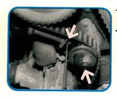
Another method is to loosen the tensioner pivot bolt. Grab your large adjustable pliers and compress the spring on the tensioner. Once you've compressed the spring, you'll see this drilling in the shaft. Slide a small allen key or drill bit into the hole to keep the spring compressed.
