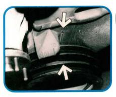
If we take time now to set the engine for TDC on number one cylinder, we'll have everything properly timed to install the new belt. If the old belt isn't broken, turn the engine until the notch on the crankshaft pulley is aligned with the zero degree reference mark on the lower timing belt cover.
