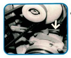
Loosen the pinch bolts on the support brackets and back off the tensioner bolt as shown. Swing the compressor toward the engine and remove the belt. The tensioner bolt for the alternator is located beneath it, just above the bolt for the compressor. Remove the alternator and compressor belts.
