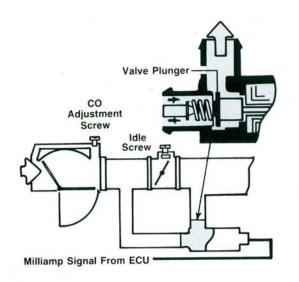
the stabilizer valve is also directly controlled by the ECU. The ECU supplies a variable milliamp current to the stabilizer valve to provide a stable engine idle speed under different load conditions.
