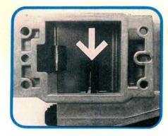
The negative temperature coefficient (NTC) air temperature sensor (arrow) is located in the inlet side of the air flow sensor. The air temperature sensor is permanently attached to the air flow sensor, so the air flow sensor must be replaced if the temperature sensor fails.
