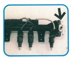
The fuel rail, pressure regulator, and injectors are combined in a compact package. The fuel pressure regulator (arrow) maintains system pressure at 2.5 bar at idle and up to 3.0 bar under full engine load. The system should hold 2.0 bar residual pressure for 15 minutes after engine shutdown.
