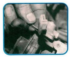
REASSEMBLY TIP TWO: We said earlier that it was pretty hard to get the engine harness connected wrong since the connectors are all different. But the connectors for the engine temp sensor and the vacuum control solenoid are similar. The one without the lock tab goes to the temperature sensor.
