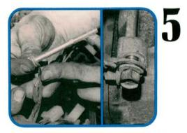
There are two main grounds bolted to the engine. One is in the engine harness and bolts to the engine at the right front intake manifold bolt. The other comes from the main battery ground and bolts to the front of the right cylinder head near the air cleaner preheat tube. Check for corrosion at both.
