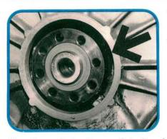
If you're replacing the crankshaft seal, you won't need the puller since you can drive the old pilot bearing out from the back with the flywheel removed. The flywheel will bolt on only one way, so you don't have to mark it. A slide hammer with a small metal screw screwed into the old seal works well as a seal puller.
