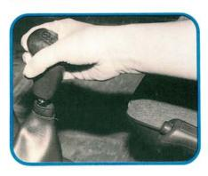
REASSEMBLY TIP ONE: Make sure the clutch disc is really on center as you tighten the clutch cover bolts. The fit between the input shaft and pilot bearing is a close one. Then select fifth gear and pull the handbrake to hold the input shaft. That way you can rock the crankshaft with a wrench until the clutch splines.
