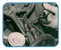
Fuel inlet and return, fuel vapor, brake booster, and heater hose connections are all located on the left side of the engine compartment. The hoses are different sizes, so you won't need to mark anything for reinstallation. Just match hose sizes to the correct size steel tubing.
