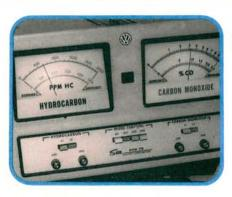
Reinstall the dipstick and remove the crankcase breather hose clamp. Set the base idle speed to 975 RPM ± 50 RPM. Reconnect the coolant temperature sensor. The idle speed should drop to 800 RPM  $\pm$  50 RPM. CO must be 0.7 percent ± 0.4 at any altitude. If idle speed is out of specs, check the stabilizer valve.
