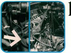
Don't take any chances with your test connections. This coil terminal jumper wire (left photo) is shielded at one end, preventing accidental grounding. The tachometer lead is attached safely inside the plastic shield. An elastic cargo strap (right photo) keeps test leads out of harm's way.
