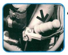
Attach an approved silicone test hose to the CO tap (arrow). Raise the oil dipstick, then clamp the breather hose near the crankcase emission control valve. Adjust the idle speed to 800 RPM ±50 RPM, then check the CO. CO will vary with altitude, because the temp sensor is disconnected, keeping the system in open loop.
