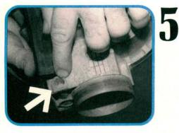
To adjust CO, carefully drill a 2.5 mm hole in the air flow sensor's tamper-proof plug. Thread a 3 mm sheet metal screw into the hole. Then remove the screw and plug using pliers. The adjustment screw takes a 5 mm hex wrench. Clockwise richens the mixture. Replace the plug when you're finished.
