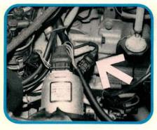
If the timing didn't advance, check the knock sensor system. Torque the knock sensor to 15-25 Nm, then check its wiring (arrow) to the ECU. Check the temp sensor's resistance, then check its wiring to the ECU. If no defects are found, substitute a known good knock sensor. If the problem continues, replace the ECU.
