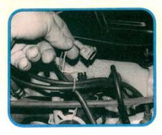
To adjust the ignition timing, start the engine and rev it four times as described in the introduction. Remove the coolant temperature sensor's blue connector to put the system into open loop. The black connector on newer models connects to the coolant temperature gauge.
