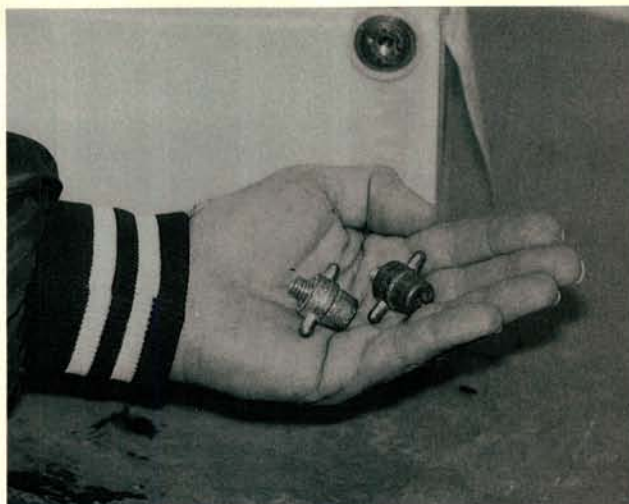
Side Terminal Lead Adapters For Load Testing Batteries. Don't use bolts.
