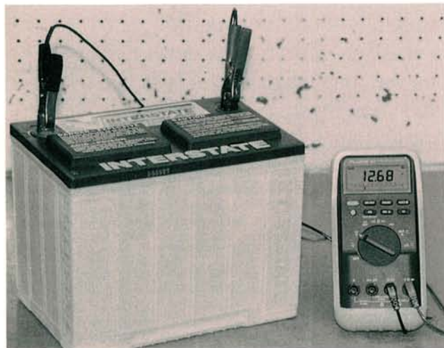
Checking Battery Terminal Post Voltage With A High Quality DVOM. Compare the reading to the "Voltage Vs. State Of Charge" chart. This test can be done either in or out of the car.
