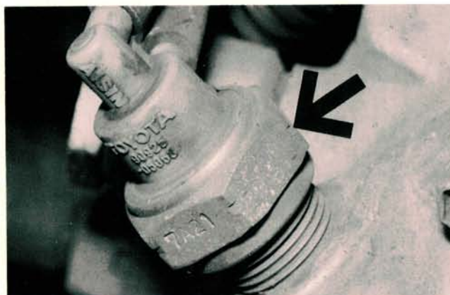
Known to nest near wetlands, Thermal Vacuum Valves spend their lives half submerged in coolant.
