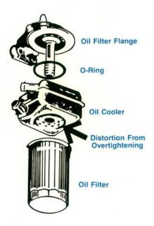
The aluminum oil cooler housing used on Volkswagen 16-valve engines can be distorted by over tightening of the oil filter during an oil change. This distortion will leave a warped sealing surface between the face of the cooler and the oil filter o-ring. High oil pressure at engine start up has blown the oil filter seal on a number of the engines as a result of this distortion.
